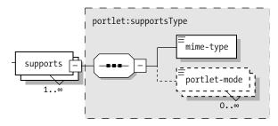
Figure 6-4. The <supports> XML Schema
