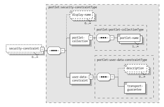
Figure 6-11. The <security-constraint> XML Schema
