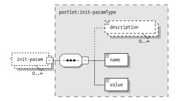
Figure 6-3. The <init-param> XML Schema
