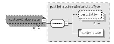
Figure 6-9. The <custom-window-state> XML Schema
